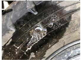
again and after giving it a thorough check with some bubble water, we indeed find the leak. That means we have to again go back to a tire repair shop...
