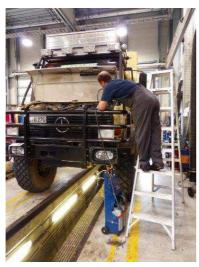
One cylinder is de-installed, the seals inside look quite ok. So the cylinder air was again drained out of the clutch system at two different points.
